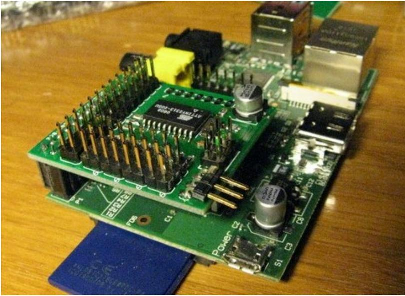
Make sure the the 2x13 female header on the servo board align in both directions with the 2x13 pin header on the Raspberry pi.
